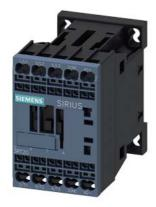
power contactor, AC-3e/AC-3, 7 A, 3 kW / 400 V, 3-pole, 24 V DC, 0.7-1.25 $^{\circ}$  Us, with integrated suppressor diode, auxiliary contacts: 1 NC, spring-loaded terminal, size: S00, suitable for PLC outputs, not expandable with auxiliary switch
